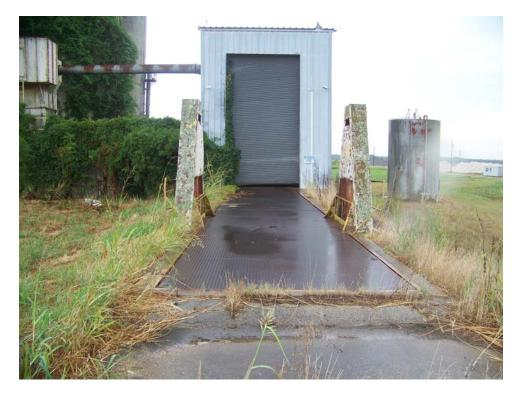
Photograph 15. Truck lift and dump
