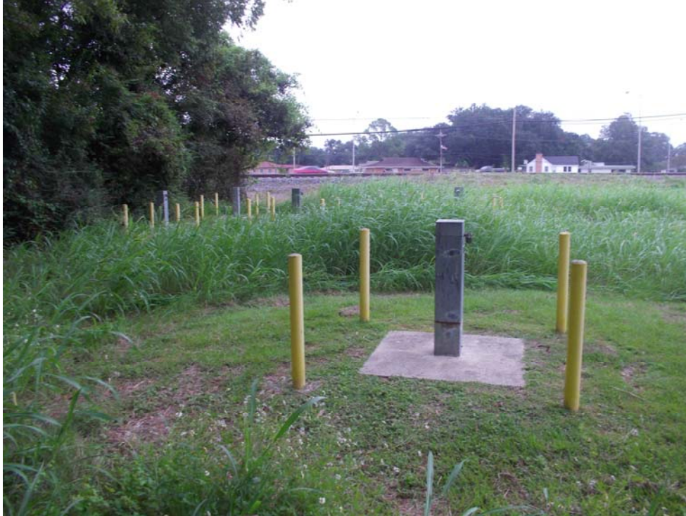
Photograph 15. Monitoring wells and railroad adjacent to southeastern corner of property
