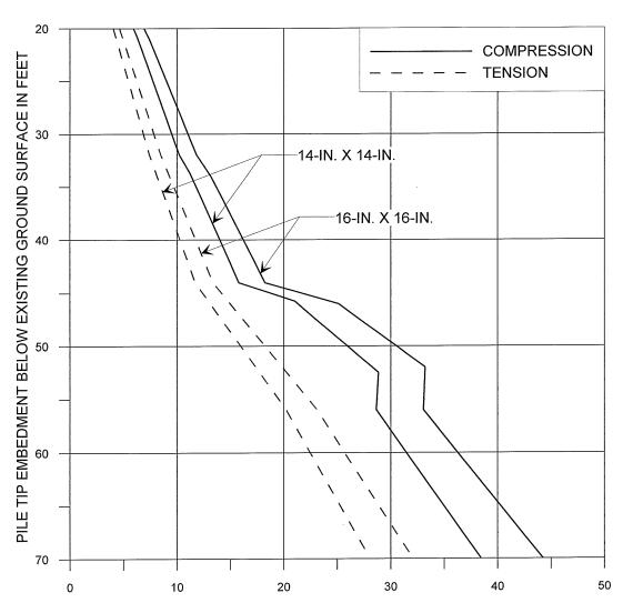
ESTIMATED ALLOWABLE SINGLE PILE LOAD CAPACITY IN TONS (F.S.  $\approx 2$ )
