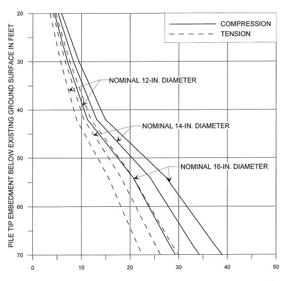
ESTIMATED ALLOWABLE SINGLE PILE LOAD CAPACITY IN TONS (F.S. ≈ 2)
